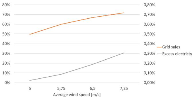
Fig. 7. Comparison of excess electricity and grid sales as a function of yearly average wind speeds. The Grid sales use the left axis while the excess electricity uses the right axis.
