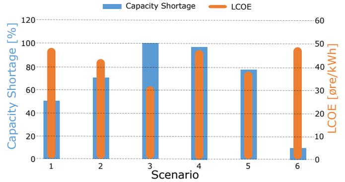
Fig. 5. Capacity shortage and Levelized cost of energy (LCOE) for each scenario.
