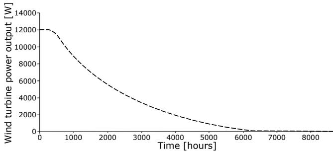
Fig. 4. Duration curve for the power output of the wind turbines over the year [10].
