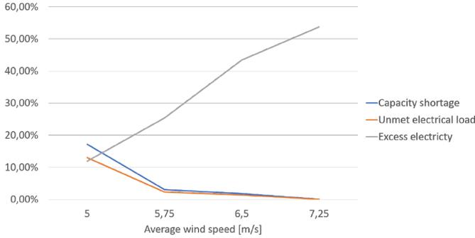
Fig. 6. Comparison of capacity shortage and excess electricity as a function of yearly average wind speed.
