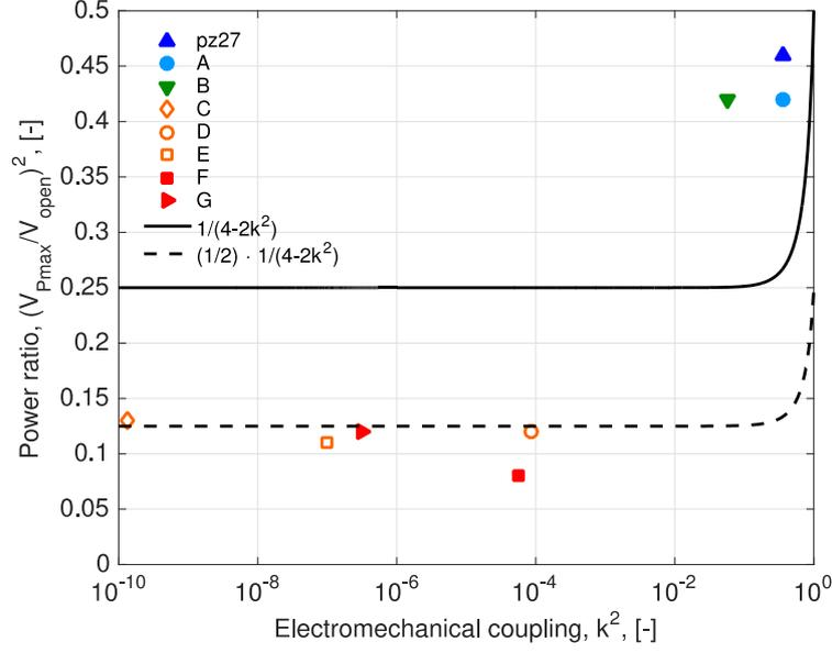
**Figure 5.** Maximum output energy over stored electrical energy in open circuit conditions as a function of electromechanical coupling coefficient,  $k^2$ . The solid line is calculated as  $1/(4-2k^2)$ , while the dashed line is calculated as  $(1/2) \cdot 1/(4-2k^2)$ .
