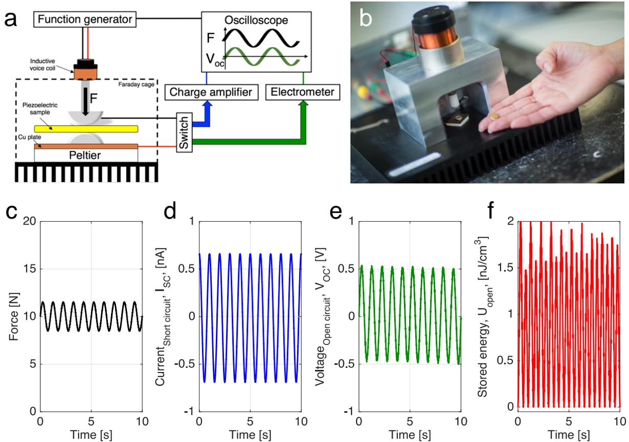
**Figure 1.** Developed piezometer system. (a) Schematic representation of the measurement system. (b) Picture of the jig. (c) Example periodic input waveform of the applied force with a sinusoidal excitation of 1 Hz. (d) The short circuit current,  $I_{sc}$ , due the sinusoidal excitation shown in (c) of a PZ27 ceramic disk. (e) The corresponding open circuit voltage,  $V_{oc}$ . (f) The corresponding stored electrical energy, per unit volume,  $U_{open}$ .
