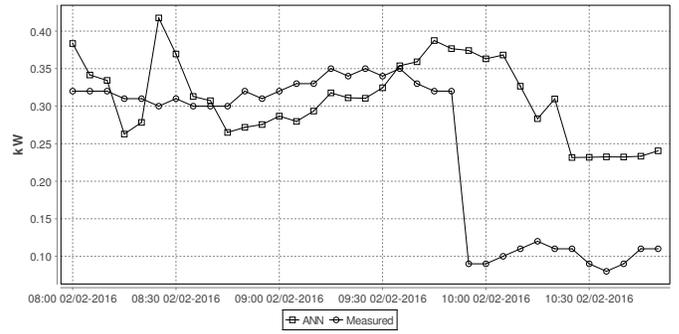
Fig. 7. Load forecasting results for the ventilation system.
