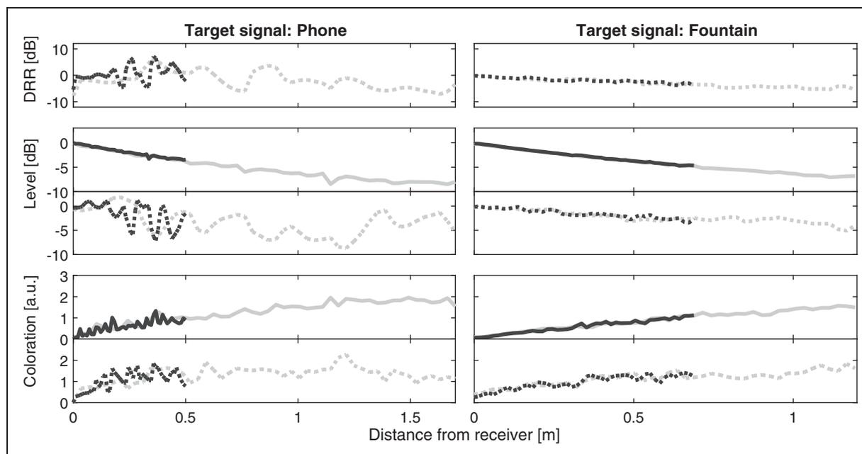
**Figure 6.** Left: changes in DRR (top), overall level (middle), and spectral coloration (bottom) for the phone signal moving either 0.5 m (black) or 1.7 m (gray) away from the listener over 2.3 s. Changes in overall level and spectral coloration are shown for both anechoic (solid lines) and reverberant (dashed lines) conditions. Right: corresponding plots for the fountain signal moving either 0.7 m (black) or 1.3 m (gray) away from the listener.
