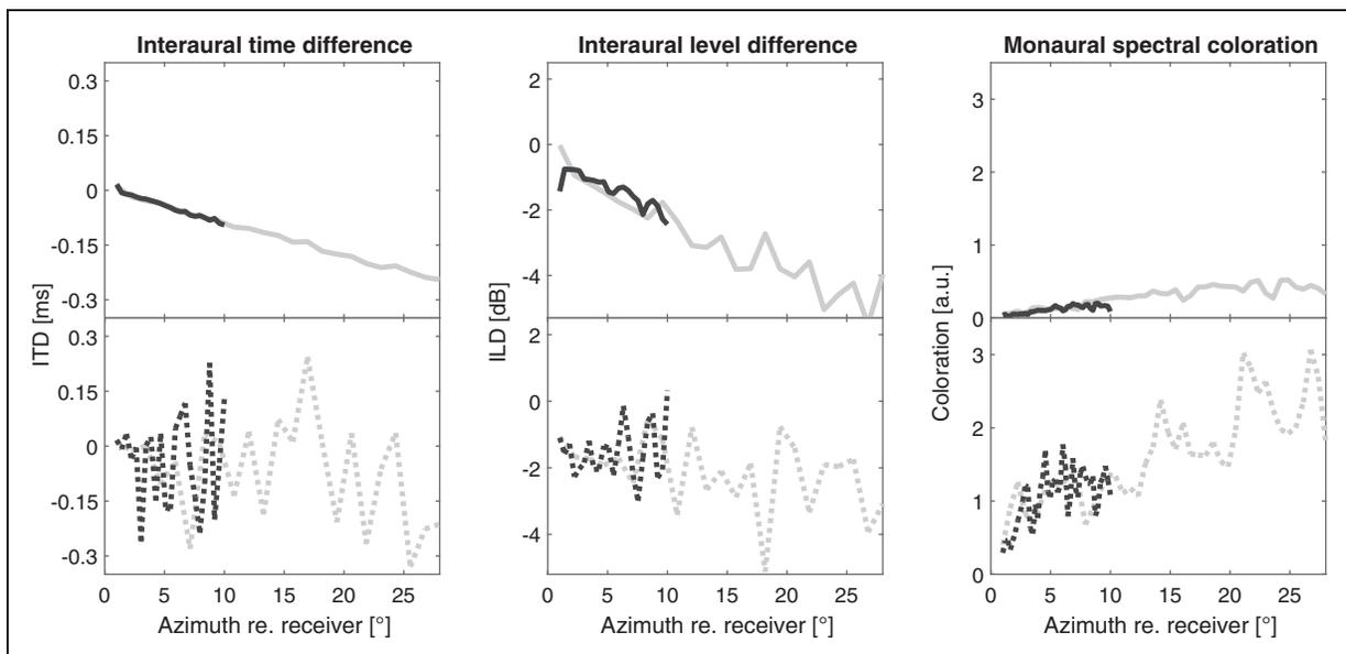
**Figure 5.** Changes in ITD (left) and ILD (middle) under anechoic (top, solid lines) and reverberant (bottom, dashed lines) conditions for the phone moving either 10° (black) or 28° (gray) to the side over 2.3 s. Monaural spectral changes (right) as estimated using the measure of Moore and Tan (2004) are also shown.
