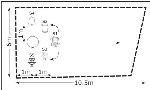
**Figure 2.** Schematic top-down view of the simulated room, showing the virtual listener and the five sound sources at  $0^\circ$  (S1),  $\pm 45^\circ$  (S2, S3), and  $\pm 90^\circ$  (S4, S5). S1 could move in the left-right/right-left or the near-far direction (see text for details).
