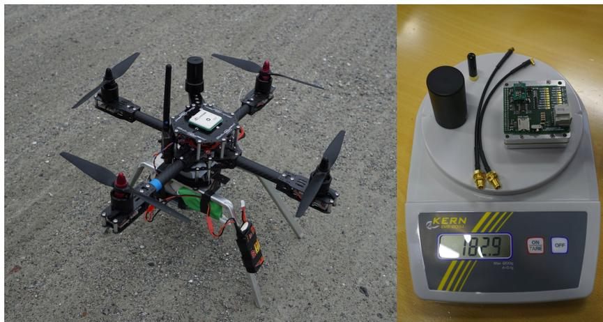
Figure 1: (a) The EduQuad drone used in this work. (b) Trimble BD920 RTK GNSS with the external interface board. The total weight including the GNSS antenna, a small stubby GSM antenna and antenna cables is 183 g.
