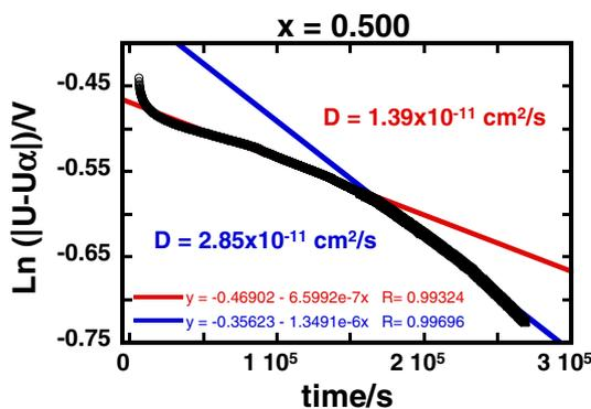
**Figure 7.** Fitting the depolarization cell voltage at point  $x = 0.5$  of Figure 6a with Eq. 1 in order to extract the chemical diffusivity. Two slopes are clearly fitted.
