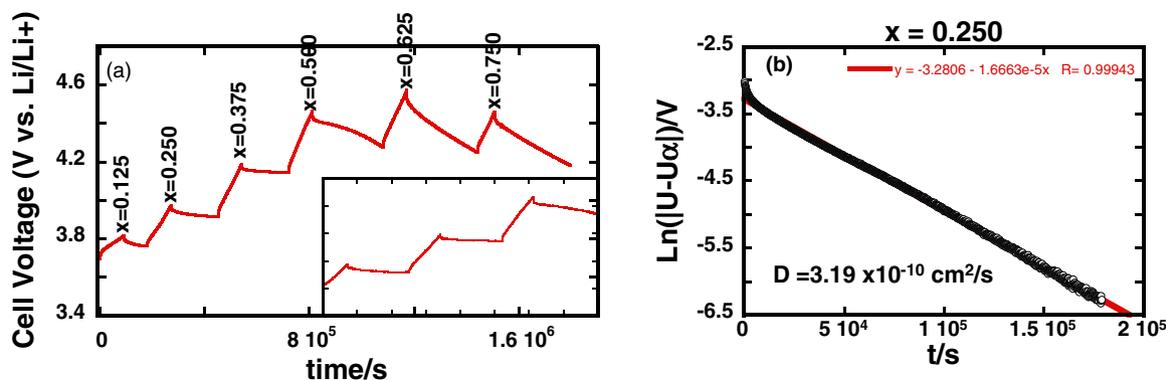
**Figure 6.** (a) Time dependent cell voltage measured on the NCA ( $\text{Li}_{1-x}\text{Ni}_{0.8}\text{Co}_{0.15}\text{Al}_{0.05}\text{O}_2$ ) plate by titrating a fixed amount of lithium and holding at open circuit conditions. (b) Fit of the depolarization cell voltage to Eq. 1 in order to extract the chemical diffusivity of lithium ion at  $x = 0.25$ .
