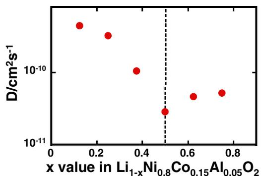
**Figure 9.** Diffusivity of NCA ( $\text{Li}_{1-x}\text{Ni}_{0.8}\text{Co}_{0.15}\text{Al}_{0.05}\text{O}_2$ ) as a function of lithium content at room temperature obtained from depolarization experiments shown in Figure 6a.
