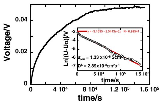
**Figure 5.** Time dependent DC polarization voltage at  $\sim 60^\circ\text{C}$  obtained from the electron blocking cell Li/PEO/NCA/PEO/Li. Results are fitted with Eq. 1 in order to obtain ionic conductivity and diffusivity (inset).
