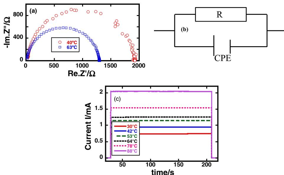
**Figure 2.** (a) Impedance spectra of as-sintered fully lithiated NCA at two different temperatures measured using the symmetrical cell configuration Ag/NCA/Ag, (b) equivalent circuit used to evaluate the impedance spectra, and (c) time dependent current in polarization measurements performed at various temperatures in the same cell configuration under constant applied voltage.
