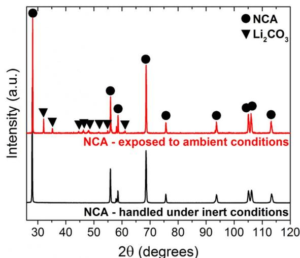
**Figure 1.** PXD data of NCA samples handled under inert conditions (black curve) and exposed to ambient conditions for 48 h (red curve), respectively. Note that  $\text{Li}_2\text{CO}_3$  is observed for the sample exposed to ambient conditions, while only peaks from NCA are observed for the sample handled under inert condition.
