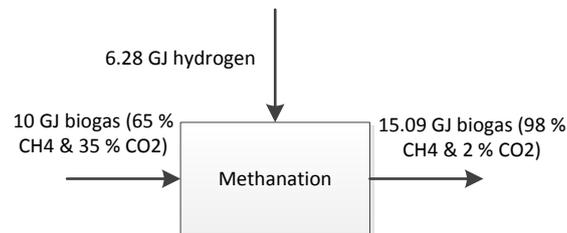
Diagram 1: Energy balances of the methanation of biogas [18]
