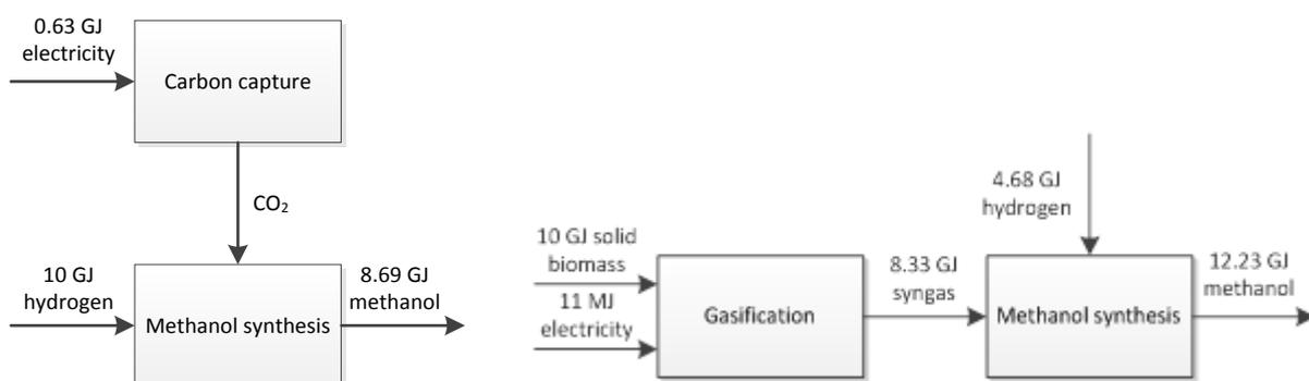
Diagram 2: Energy balances of hydrogenation of syngas and captured carbon dioxide [1,9]
