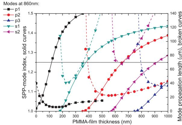
Fig. 2. Calculated effective mode index (solid curves) and mode propagation length (broken curves) for the first three  $p$ -polarized hybrid plasmonic modes (p1, p2, p3) and the first two  $s$ -polarized photonic modes (s1, s2) existing in a four-layer structure: air/PMMA/50-nm-gold/glass.
