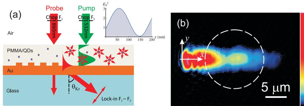
Fig. 1. (a) Experimental configuration. Thin PMMA film doped with PbS quantum dots on top of a 50-nm-thick gold film. Excitation of a probe SPP beam ( $\lambda = 860$  nm) is achieved through a grating. Inset shows a calculated distribution of the intensity of the pump beam ( $\lambda = 532$  nm) inside the PMMA layer. (b) Leakage-radiation microscopy image of a probe SPP beam. The dashed circle shows the position where the pump beam is focused.
