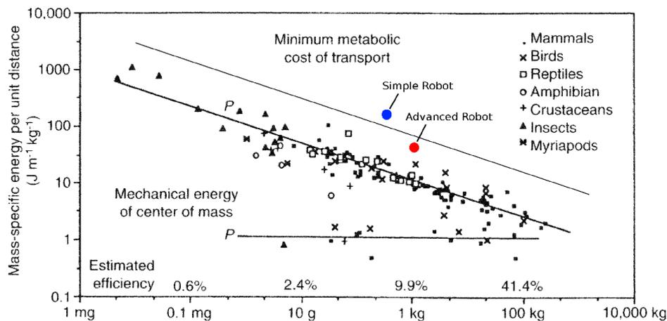
**Figure 1:** The graph shows the cost of transport plotted against the weight of various animals, together with the COT values for the two robots - (red) advanced robot, (blue) simple robot. The horizontal line marked "P" tells the mechanical cost of transport of some animals, and not used in this work. Full et. al [1]
