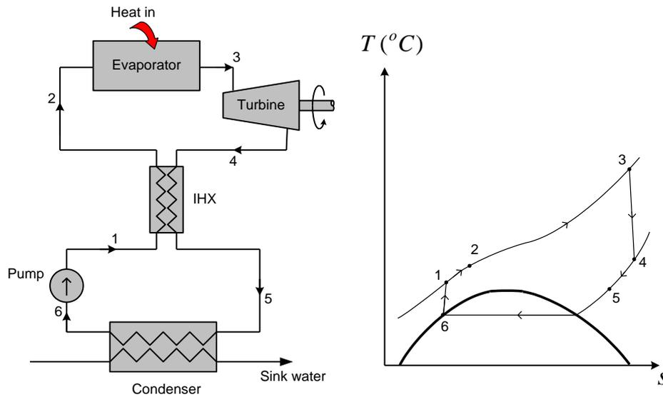
Figure 1. Left: The generic configuration for the Transcritical Rankine Power Cycle (TRPC). Right: Cycle in T-s diagram with corresponding state points.
