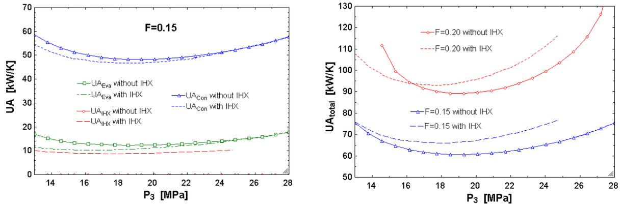
Figure 6. Left:  $UA$ -value for each of the three heat exchanger with and without IHX for  $F = 0.15$ . Right: Total  $UA$ -value for all heat exchangers with and without IHX for  $F = 0.15$  and for  $F = 0.20$ .
