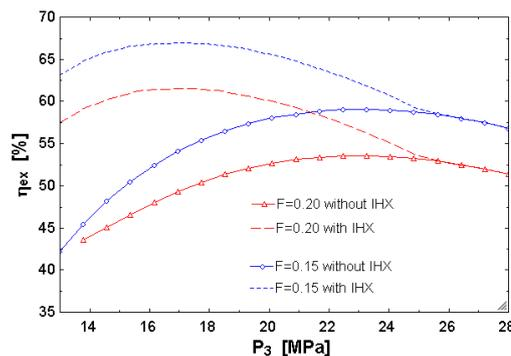
Figure 5. Exergetic efficiencies  $\eta_{ex}$  with and without IHX for  $F = 0.15$  and  $F = 0.20$ .
