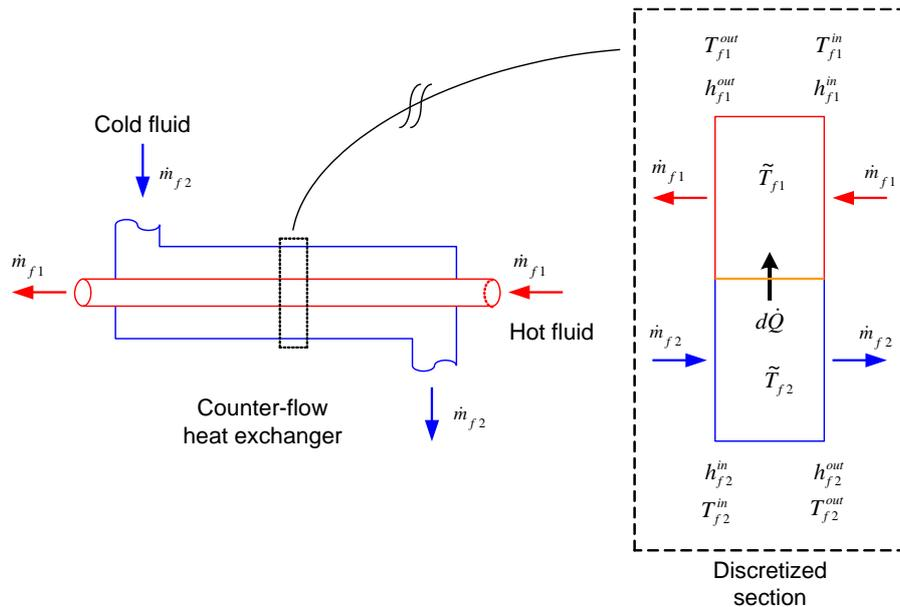
Figure 3. Discretising the counter-flow heat exchanger.
