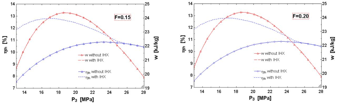
Figure 4. Left: Thermal efficiency  $\eta_{th}$ . Right: specific output  $w$  with and without IHX for  $F = 0.15$  and for  $F = 0.20$ .
