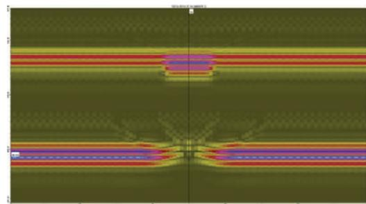
Fig. 4. B-Scan of brush 1 at 50mm (probe movement along the horizontal black line of Fig. 3, cross section over the defect).
