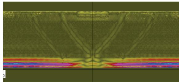
Fig. 8. Array probe at 5mm from sample, brush 1 TFM reconstruction of shallow defect (same as Fig. 2 (b), Fig. 4 and Fig. 6).
