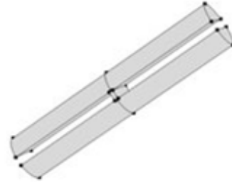
Figure 3: Geometry used in the COMSOL simulations. The diameter f and slit width w are scalable and the center bar is automatically adjusted to fill the slit.
