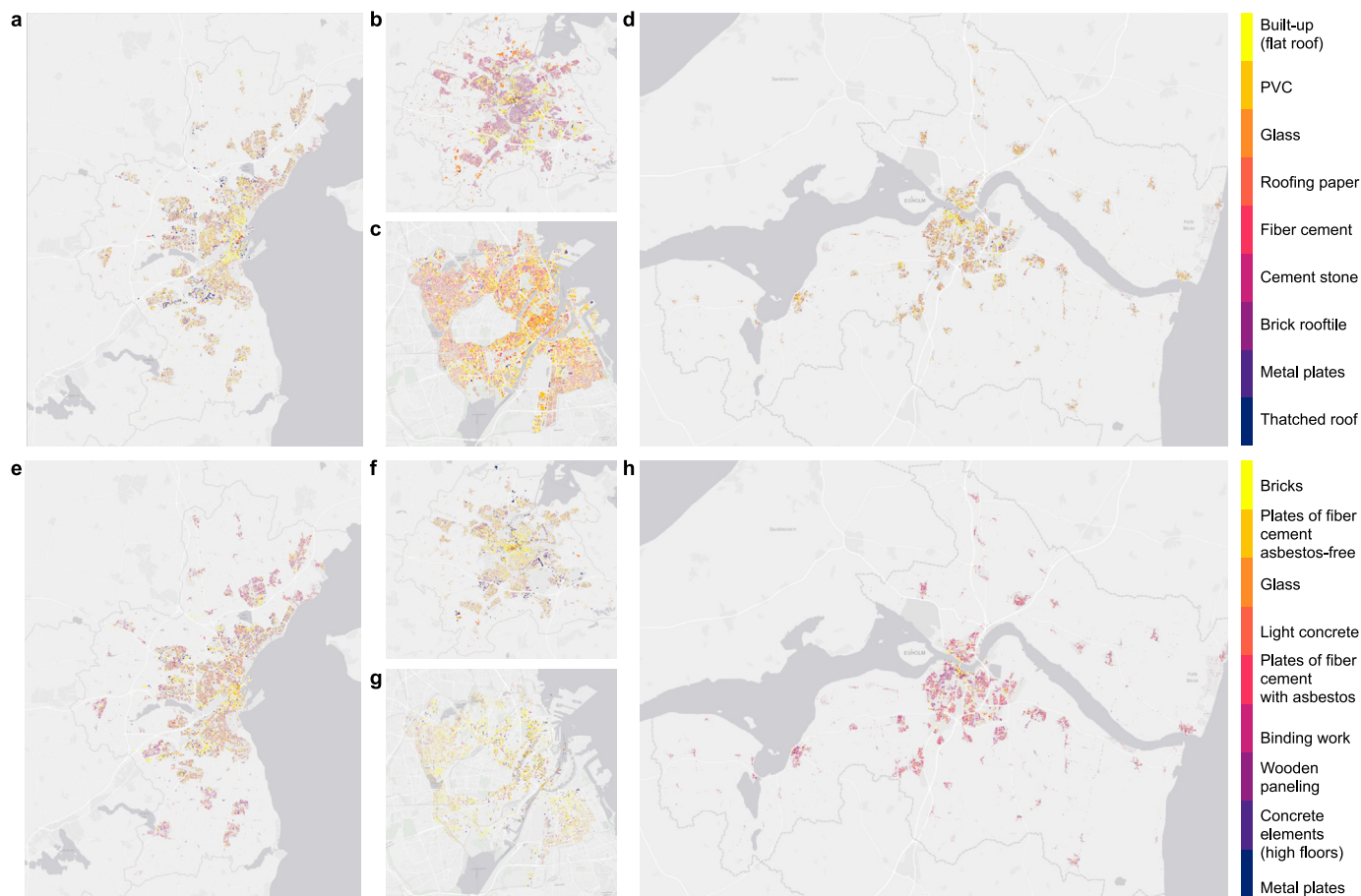
Fig. 6. a–d, The city-scale roofing classification maps of Arhus (a), Odense (b), Copenhagen (c), and Aalborg (d). The maps synthesize the results of the optimal deep learning model applied to roof images of all urban buildings, with counts of 43,476, 84,542, 59,767, and 85,902, respectively. Each building is represented by a color-coded point based on the classified roofing material, with the scale of data indicating near-complete urban coverage. e–h, Detailed predicted urban façade material distribution maps of Arhus (e), Odense (f), Copenhagen (g), and Aalborg (h), denoting each material with a color-coded marker derived from 18,571, 31,695, 26,928, and 23,916 building images, respectively. The disparity in image volumes is attributed to data unavailability and variable image quality.
