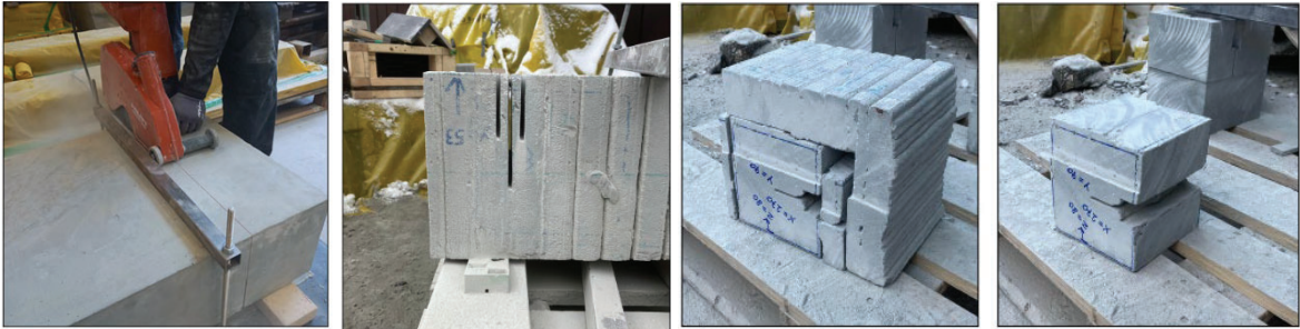
Fig. 3. Method for cutting blocks and notches for WST specimens, notches cut into specimens, and the specimen placement inside the blocks once extracted.
