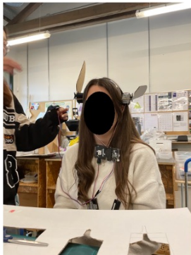
Figure 1: Head-worn interactive ears tracking and responding to the pulse of the wearer.
