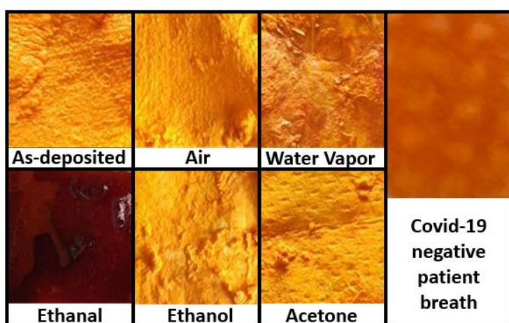
Figure 1. Images of facemask fabrics covered with ethanal-sensitive colorimetric solutions. The masks were exposed to several gases for 8 h. A clear change in color is exclusively observed upon exposition to ethanal.
