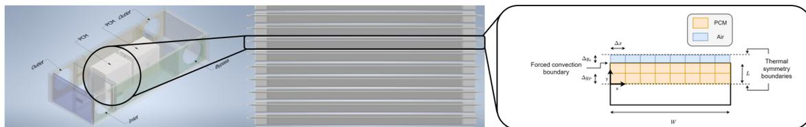
**Figure 1:** Left: 3D drawing of climate module with PCM. Middle: 2D view of the PCM plates with PCM inside them. Right: Discretization of the PCM and air into nodes.
