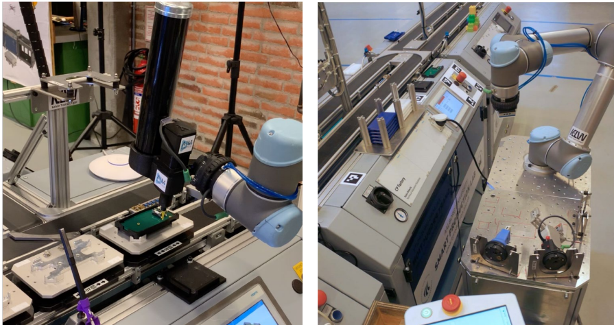
Fig. 1. The robot assistant tending the two manual workstations at AAU Smart Production Line. The robot carries generic tools on its platform, see right-hand picture. The robot also makes use of station specific tools available at the stations, see left-hand picture.
