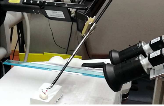
Figure 6: Laboratory setup with the da Vinci PSM, stereo camera rig and podium with marked points for needle insertion.
