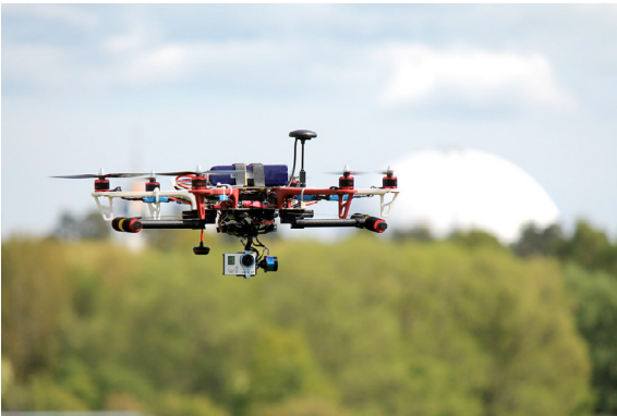
Fig. 2. Image of a hexacopter DJI F550, similar to the system simulated.
