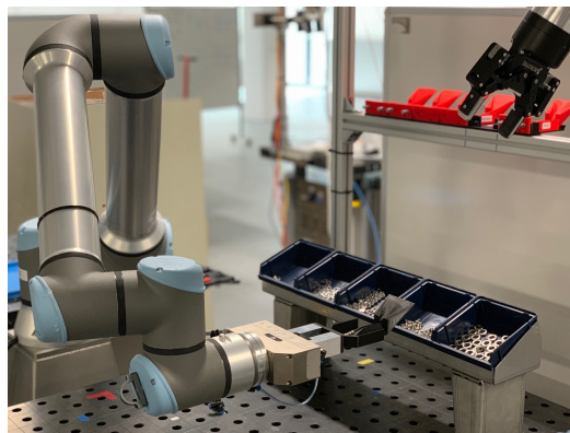
Fig. 1: The tool, or scoop , will scoop up parts from the bins and shake them until only parts in a desired orientation remain in it. Parts can then be picked from it. Thereafter, the scoop can be returned to the rack and the robot can attach another 2 .
