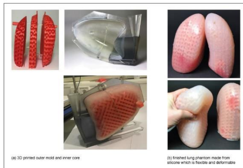
Figure 1: 3D print and finished lung phantom made of silicone
