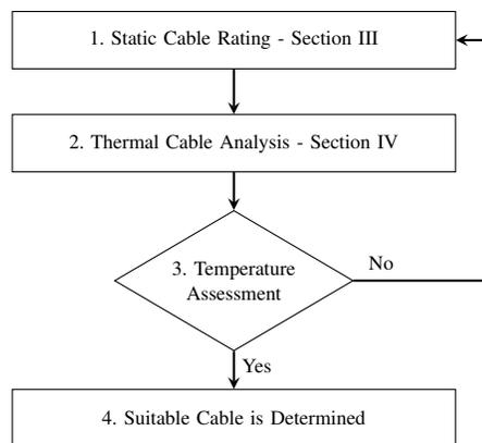
Fig. 5. Flowchart of the iterative dynamic cable rating method
