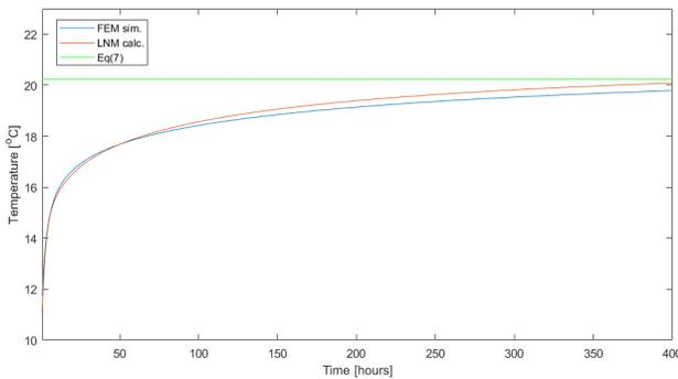
Fig. 11. Long transient response to a constant load step
