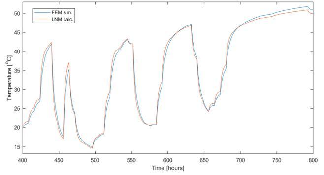
Fig. 12. Wind-based short transient response to a varying load profile
