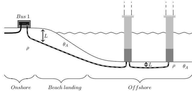
Fig. 1. Submarine cable power system from offshore wind farm and surrounding conditions
