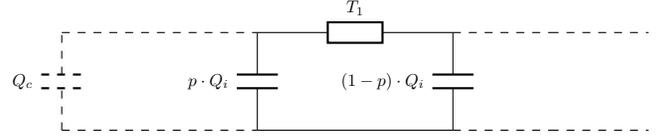
Fig. 8. Thermal representation of dielectric
