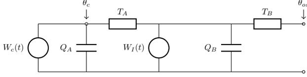
Fig. 10. Final thermal ladder network
