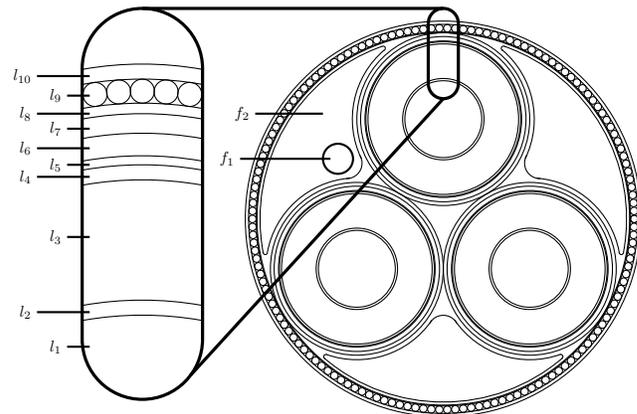
Fig. 2. Common construction of a three-core XLPE SL sheath type submarine cable
