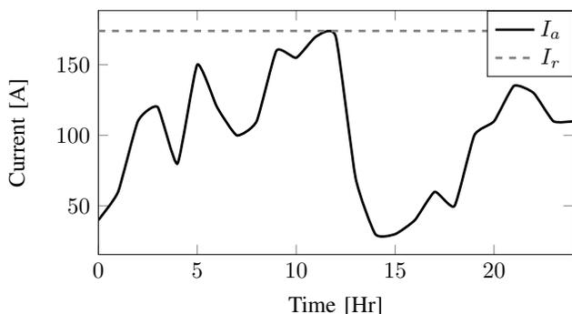
Fig. 3. Variable current profile illustrating the difference between the actual flowing current and the rated current
