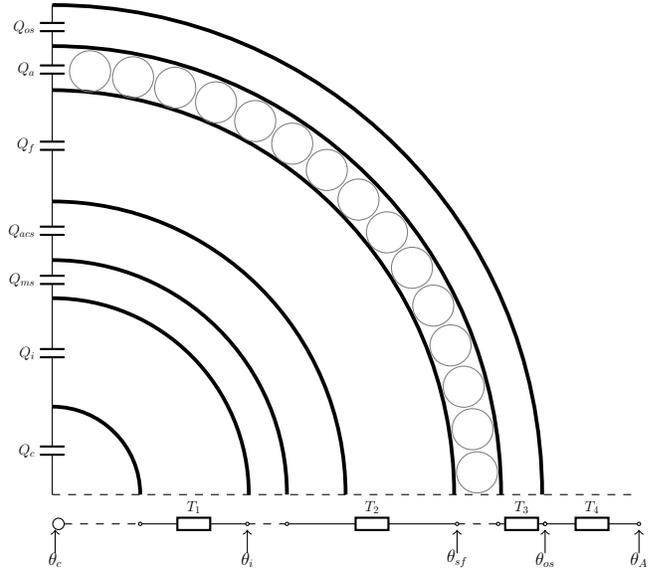
Fig. 7. Single-core XLPE SL sheath type submarine cable equivalent
