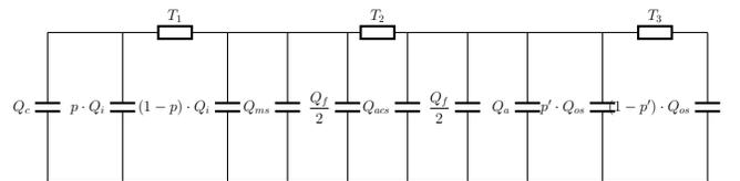
Fig. 9. Thermal three-core XLPE submarine cable ladder network
