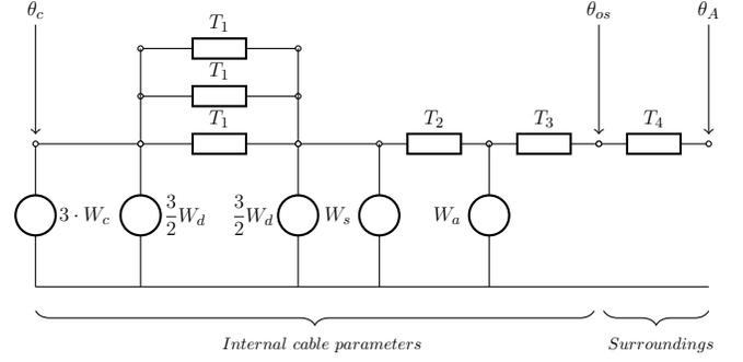
Fig. 6. Static representation of thermal resistances  $T_n$  in a three-core XLPE SL sheath type submarine cable, including power losses  $W_n$  located in the respective layers and temperature denotation  $\theta_n$
