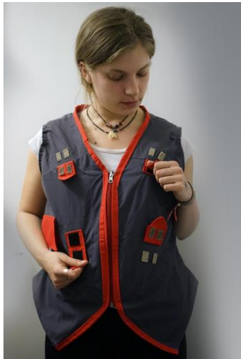
Figure 8. 2nd. Prototype, showing three open and one closed soft switch. The closed switch (under the right hand) points to the hip, where the pressure sensor is positioned.
