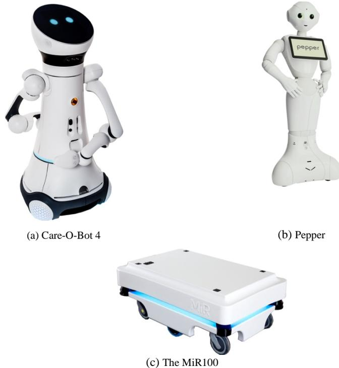
**Figure 2.** Robotic solutions for the health care system. Permission to use the figures are given by (a) Fraunhofer Institute, (b) Softbank Robotics and, (c) Mobile Industrial Robots
