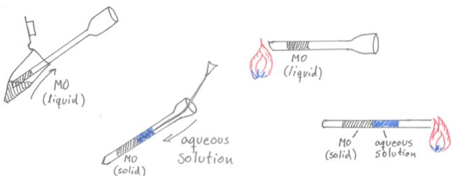
Figure 1: Procedure for preparing samples in glass capillaries.
