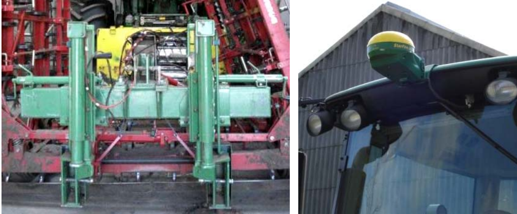
Sensor structure located in the three-point-linkage with three extended octagonal ring transducers (left). GPS receptor integrated in the tractor (right).
