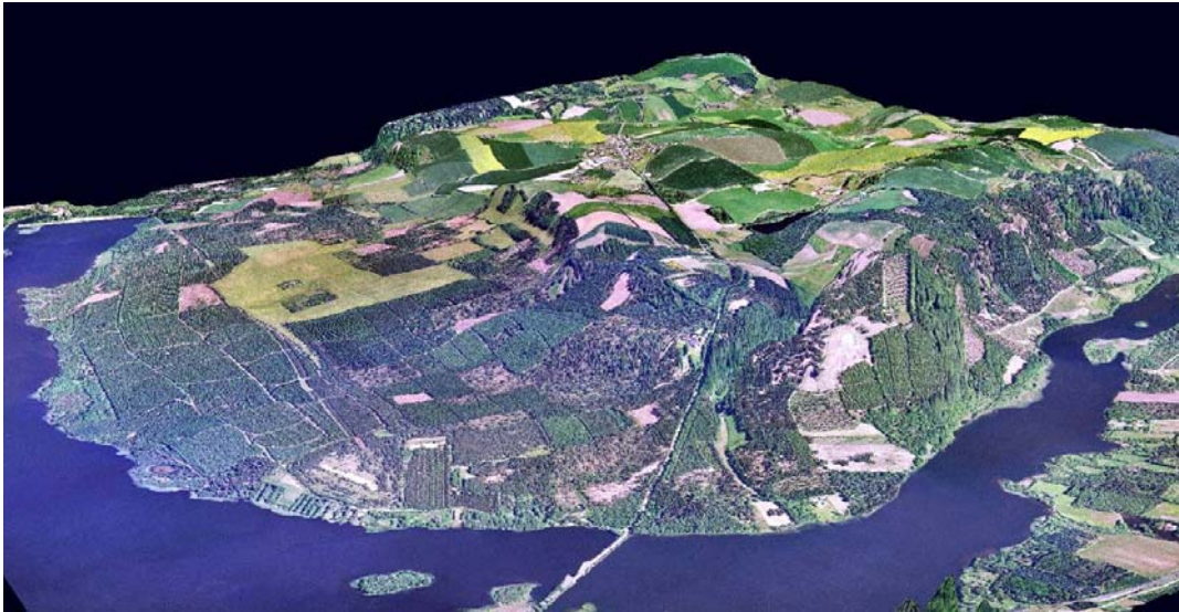
Fig 1. The study area illustrated by draping orthophotos on the LIDAR based digital elevation model.
