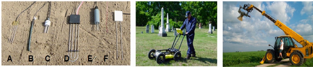
Fig.1. Some soil sensors:(A) time domain reflectometer, (B) ECH20 EC-20 probe, (C) Hydra probe,(D) Acclima time domain transmission sensor, (E) ThetaProbe, (F) CS-616. The center figure shows a cart-mounted ground penetrating radar (GPR); the right figure is a passive microwave remote sensing radiometer mounted on a crane. (Robinson et al., 2008)
