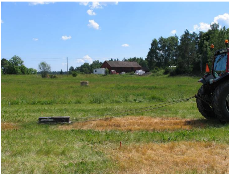
Figure 1. Measuring the electrical conductivity with a commercial soil electrical conductivity meter (EM-38; Geonics Ltd.) eight days after spreading. The grass turned into yellow in the plots with the highest nitrogen rates.
