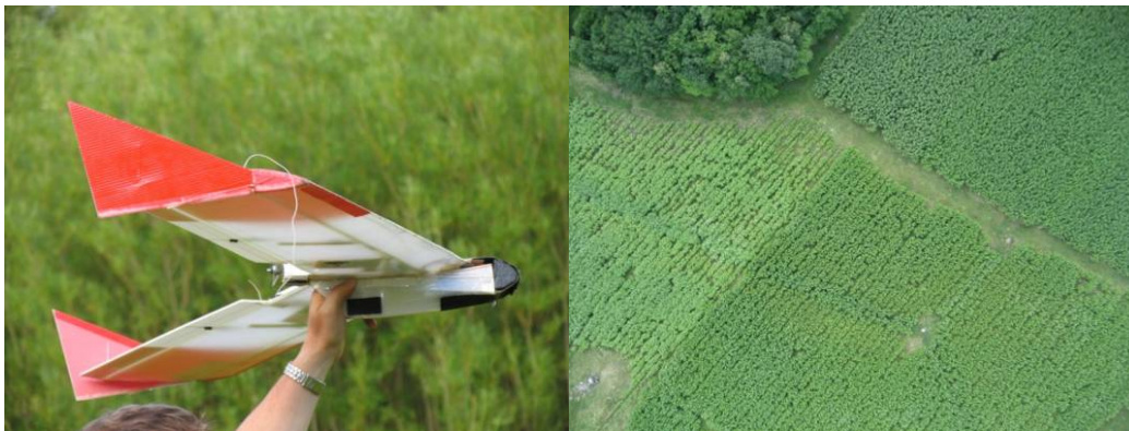
Figure 1. Left: The UAS is hand launched and controlled manually to avoid obstacles. At 50 m altitude the autopilot is engaged and navigates the aircraft according to the predefined flight route. Right: Willow fields with three varieties.
